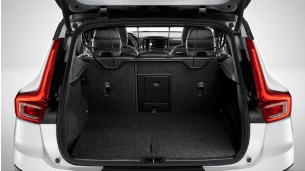
A practical protective grille that prevents loads or pets from being thrown forward into the passenger compartment in the event of heavy braking or a collision.
